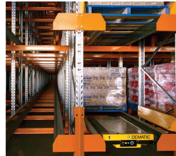
Pallet Runner Satellite Storage Maximum storage and operational effectiveness
